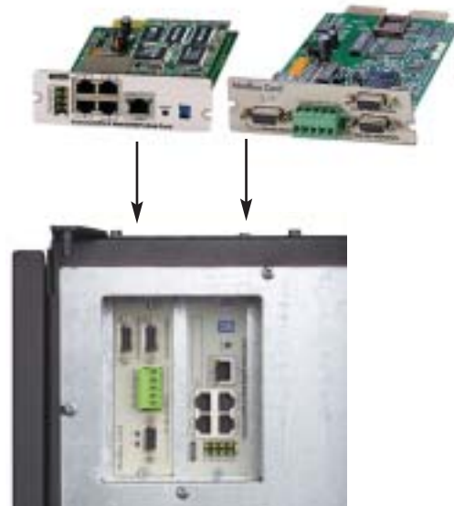
Two standard, embedded X-slots provide “plug-and-play” support for multiple communication cards. A total of four X-slots are available with the Mini-CSB option.
